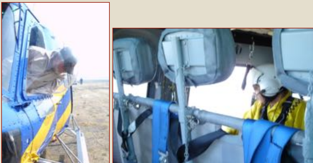
Pilot in the same type of aircraft demonstrating the proper position for longline operations (Left). View from the left seat of the helicopter, over the pilot’s right shoulder and out the right rear window, taken from a fully upright position (Right).
